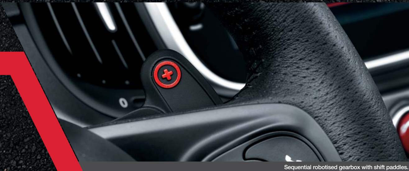
Sequential robotised gearbox with shift paddles.
